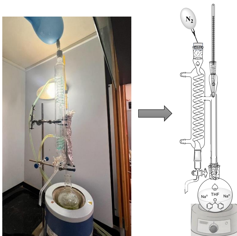
Figure 5. THF drying setup.
