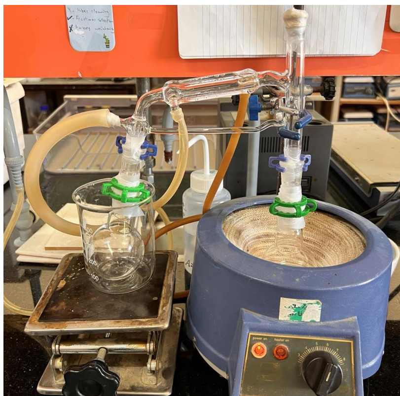
Figure 9. Distillation of boronate setup.
