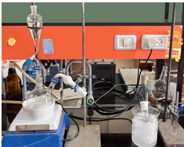
Figure 7. HCl/Et 2 O preparation setup.
